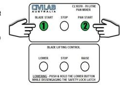
The pan drive has a "soft start" feature which is factory set. This reduces sudden starting and shock loading of the pan drive. Soft Stop is also incorporated for the same reason. This can be awkward to control during jogging operations but may assist in certain circumstances. The settings for this feature can be adjusted if required. Please refer to page 5 of the manual.
