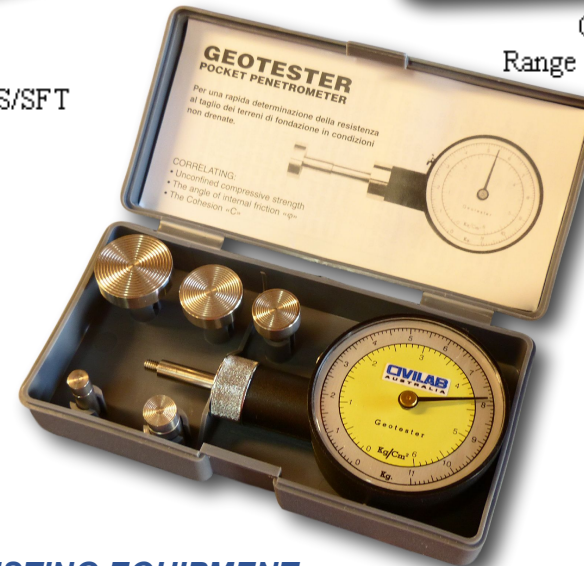
CL24565 - Geotester It has tips of 6.4mm, 10mm, 15mm, 20mm and 25mm diameter. Its outer dial reads the penetration force in kg. Its inner dial is calibrated in unconfined compressive strength for the 6.4mm tip, with the units being kg/sq. cm, which is equal to Tsf.
