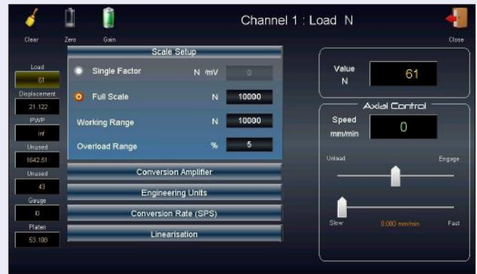
TriSCAN Advanced touchscreen display showing Load Calibration Screen
