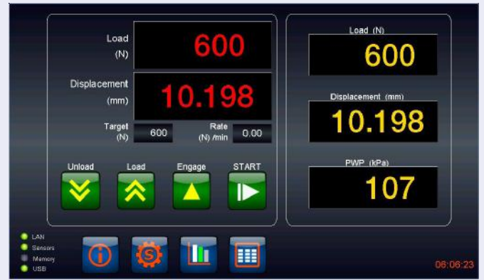
TriSCAN Advanced touchscreen display showing main details and controls.
